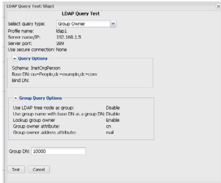
**Figure 155:**LDAP Query Test: Group Owner (Use group name with base DN as group DN is enabled)
