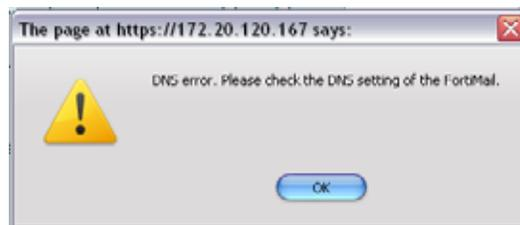
8. Verify that the DNS servers contain A records to resolve `service.fortiguard.net` and other FDN servers. To try to obtain additional insight into the cause of the query failure, manually perform a DNS query from the FortiMail unit using the following CLI command:
