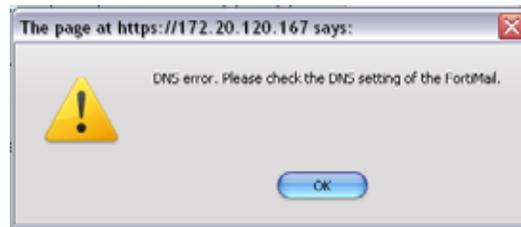
Verify that the DNS servers contain A records to resolve `service.fortiguard.net` and other FDN servers. You may be able to obtain additional insight into the cause of the query failure by manually performing a DNS query from the FortiMail unit using the following CLI command:
