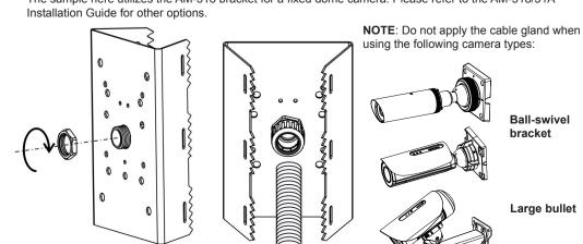
Fill the unused holes on the bracket using the included silicone stoppers. Please check the following drawings for the mounting holes and the unused holes for your models.
