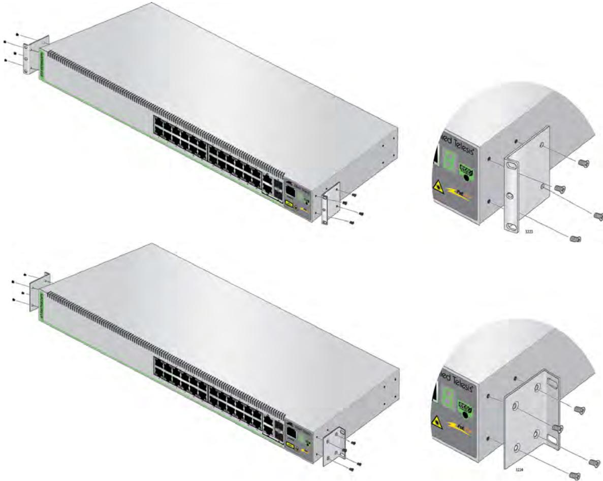
Figure 23. Attaching the Equipment Rack Brackets
