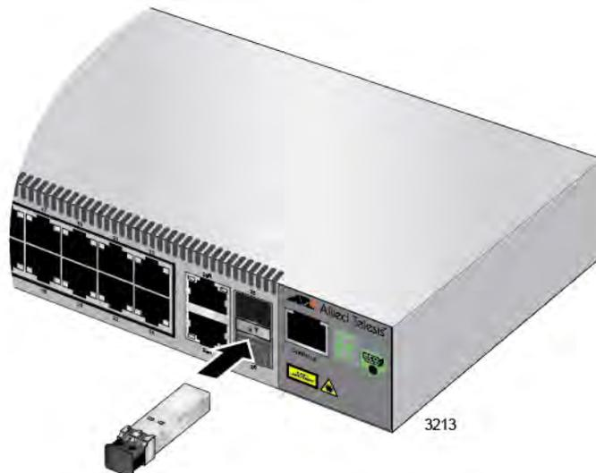
Figure 29. Installing an SFP Transceiver
