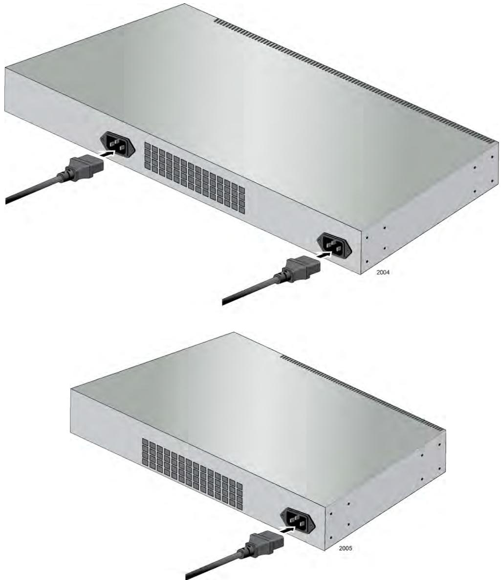
Figure 33. Plugging in the AC Power Cord
