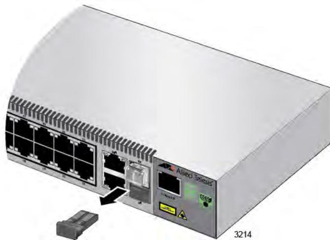
Figure 30. Removing the Dust Cover from the SFP Module
