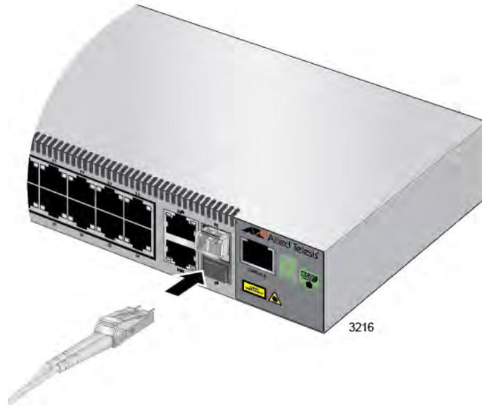
Figure 32. Connecting the Fiber Optic Cable to the SFP Module
