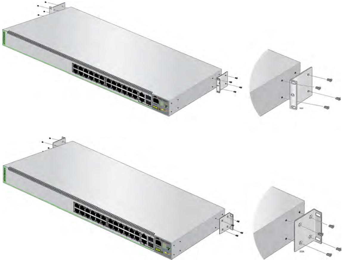
Figure 24. Attaching the Equipment Rack Brackets (Continued)
