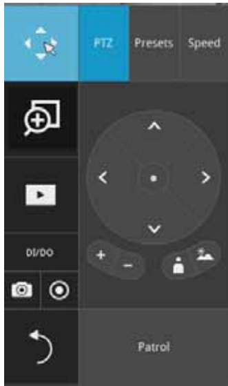
PTZ control panel for ordinary PTZ type
