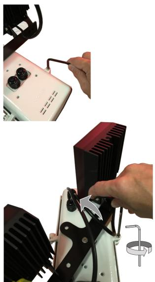
**7.** Check the inside of the enclosure to make sure the I/O wires can reach the power supply unit inside. An approximate of 25cm cable length is required. Install and tighten up the waterproof connectors.
