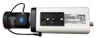
**11.** Place the mounting plate on top of the buffer pad and then secure it to the camera. You may need adjust its position so that the lens module can flush align with the tempered glass.
