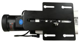
12. Secure the camera to the enclosure by securing screws through the keyhole slots.
