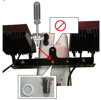
**4.** Adjust the IR lights' shooting direction and tighten up the mount screws. You may need to adjust the shooting angles later.
