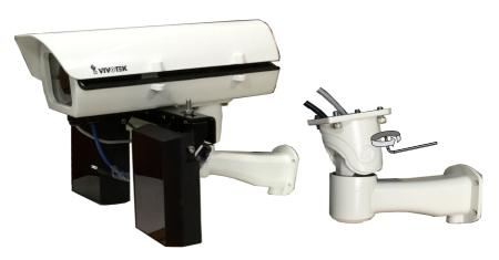
18. Adjust zoom and focus and open a web session with the camera to tune for the best image. When zoom and focus is done, Close the top cover and fasten the top cover screws.
