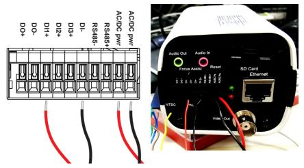
The day/night mode DO connection enables the synchronization of IR light and the automated day/night switching mechanism on the camera.
