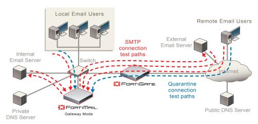
Figure 59: Connection test paths (gateway mode)
