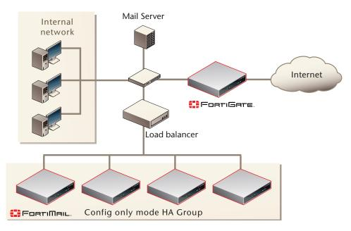
If the config-only HA group is installed behind a load balancer, the load balancer stops sending email to failed FortiMail units. All sessions being processed by the failed FortiMail unit must be restarted and will be re-directed by the load balancer to other FortiMail units in the config-only HA group.
