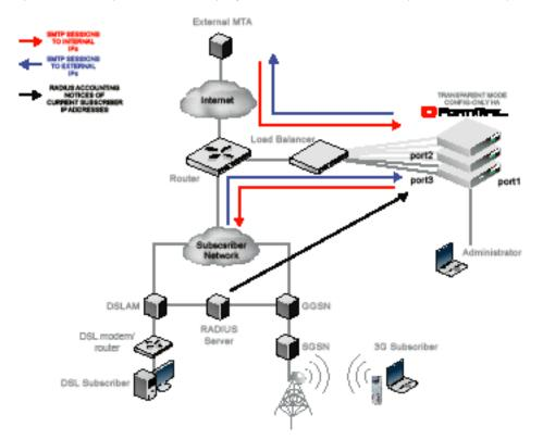
Each network interface in the dual-arm attachment (port2 and port3) is removed from the Layer 2 bridge, and is configured with its own IP address. This reduces the possibility of Ethernet loops and improves compatibility with other filtering devices.
