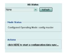
Figure 89: Active-passive HA status (primary unit after failover)
