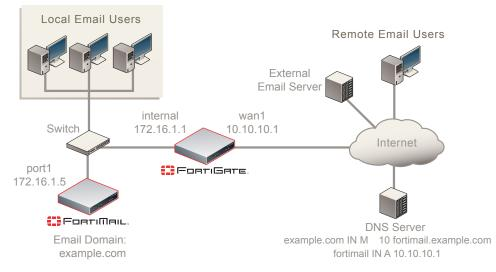
To deploy the FortiMail unit behind a NAT device such as a firewall or router, you must complete the following:
