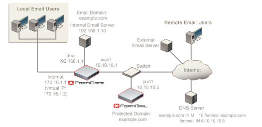
To deploy the FortiMail unit in front of a NAT device such as a firewall or router, you must complete the following:
