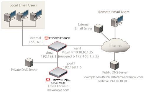
To deploy the FortiMail unit in the DMZ of a NAT device such as a firewall or router, you must complete the following:
