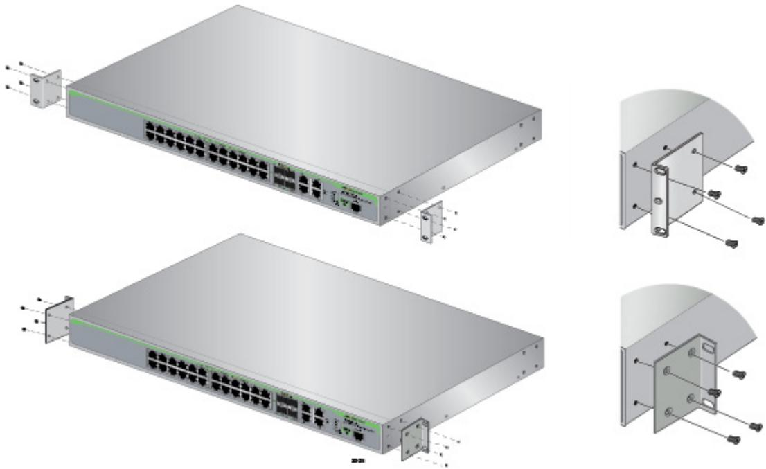
Figure 14. Attaching Brackets for Rack Mounting
